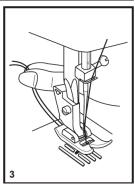
Gently pull on the upper thread to bring the bobbin thread up through the needle plate hole. (2)
